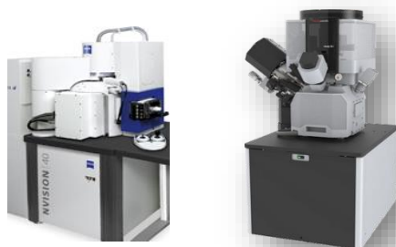
Fig. 1. Different SEM techniques to be used by students during the practical course – left : Zeiss NVision 40 with Gallium-FIB; and right : Helios 5 PFIB Cxe with Plasma-FIB.
